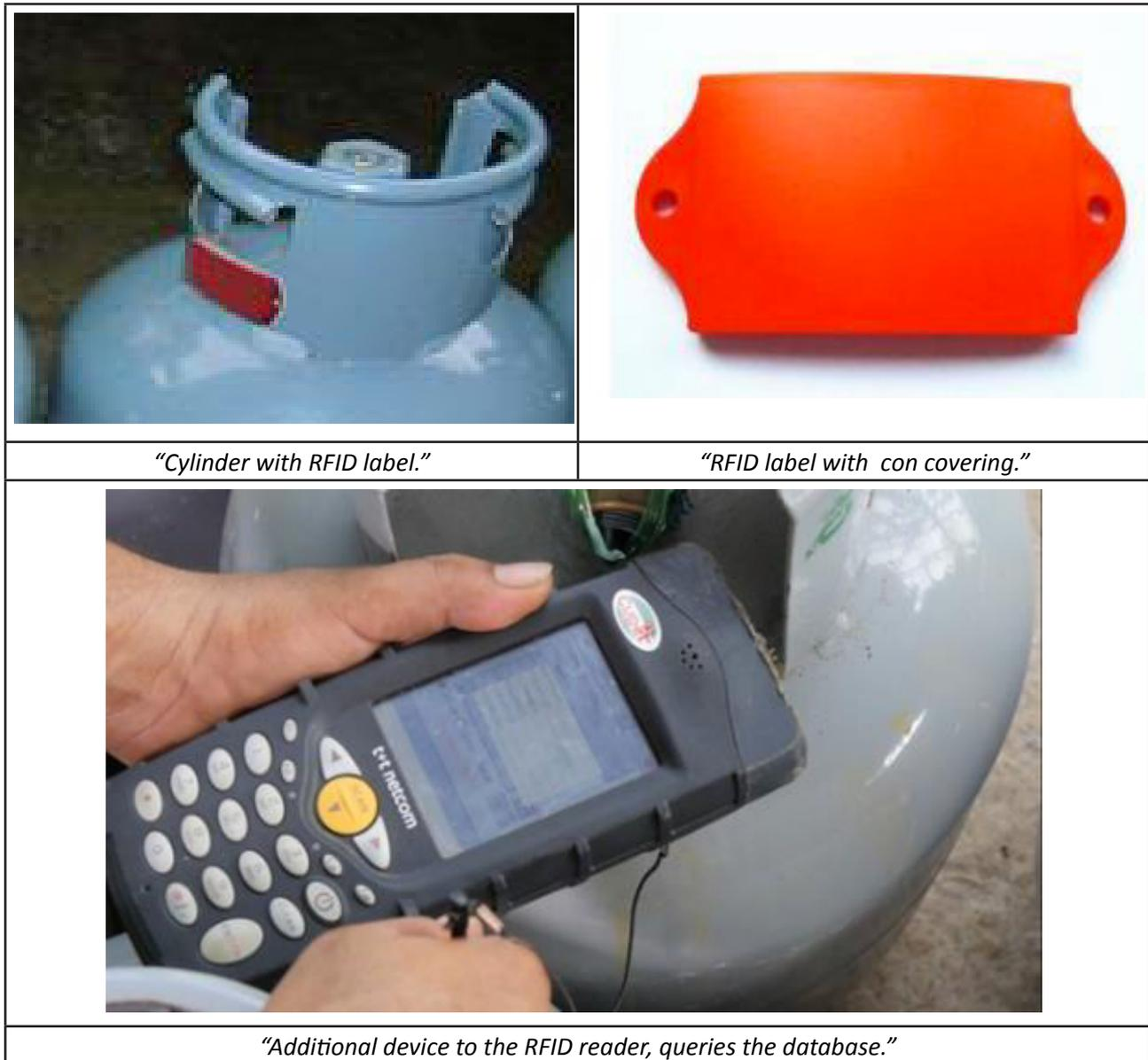
Fig3. Main elements for the implementation of gas cylinders monitoring
