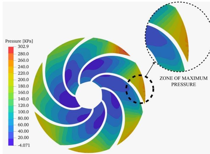
Fig. 6 Pressure contours
