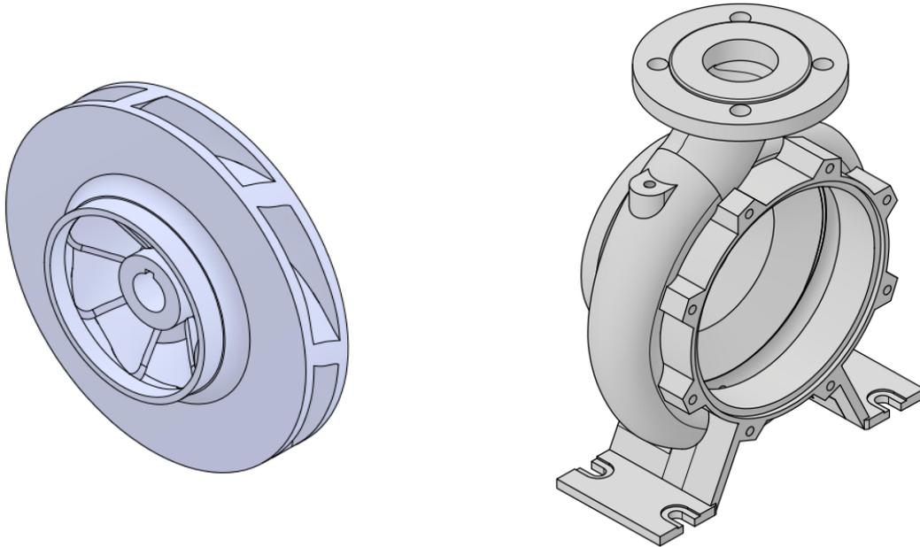
*Fig. 1 Pump impeller obtained by reverse engineering technology.*
